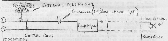
First select a suitable telephone and "get well in" with the local inhabitants. Then fix up a piece of thread along the route the loudspeaker leads are to take & measure the length of wire required. Acquire the wire, pinch the amplifier and swipe the Loudspeaker, and connect up as in diagram.
