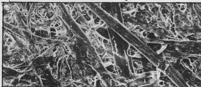
Recycled paper enlarged 100 times under an electron microscope.
