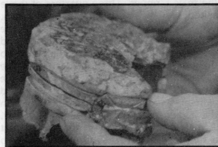
This burnt down piston was the result of an engine disintegration
