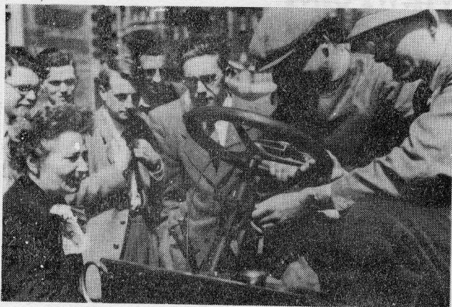
HODSON AND TROTCHAN UP - but not very far yet. Note the throttle (covered by the co-driver's hand) and the ignition lever above the steering wheel.
