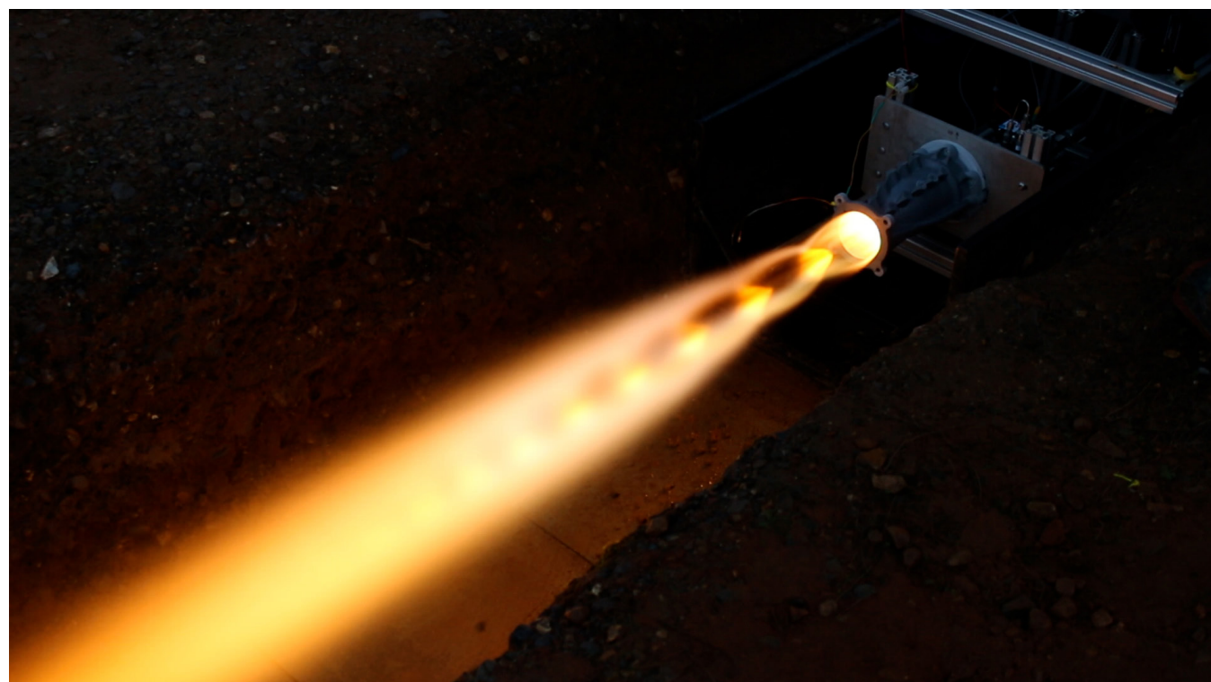
THANOS-R hot-fire test: patterns seen are called Mach Diamonds which occur as a result of shockwaves produced by the supersonic exhaust gas. The velocity of these exhaust gases is approximately 2000m/s. ICLR
