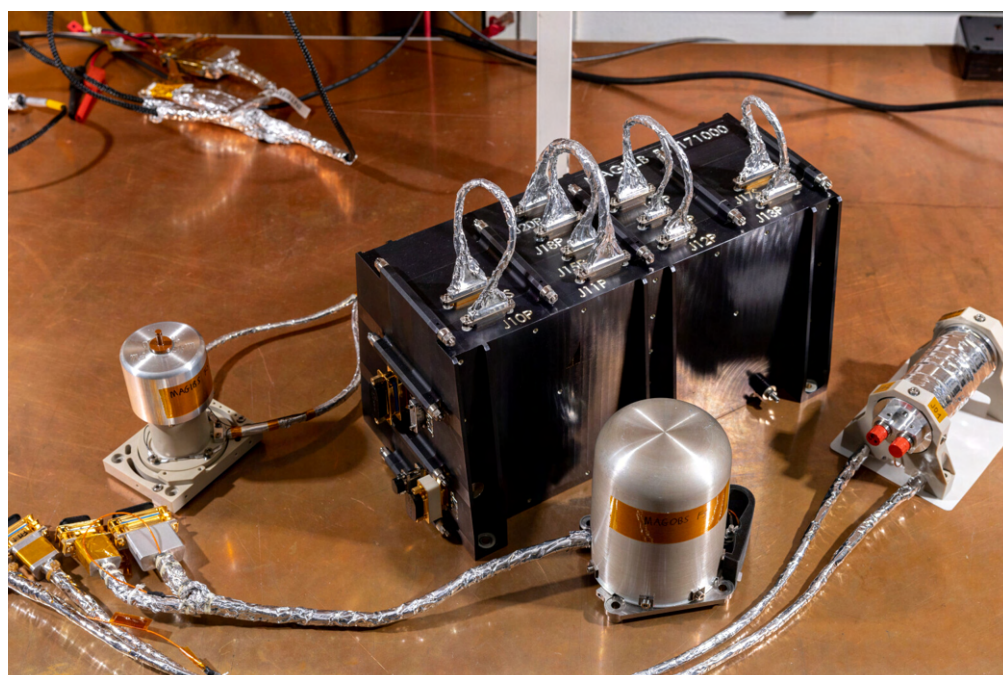
J-MAG, Imperial's magnetometer currently onboard JUICE. Imperial College London.
