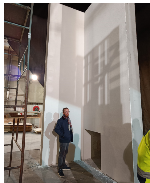
DIN 4102-20 façade fire test: before and after. Dr Matthew Bonner (left)
