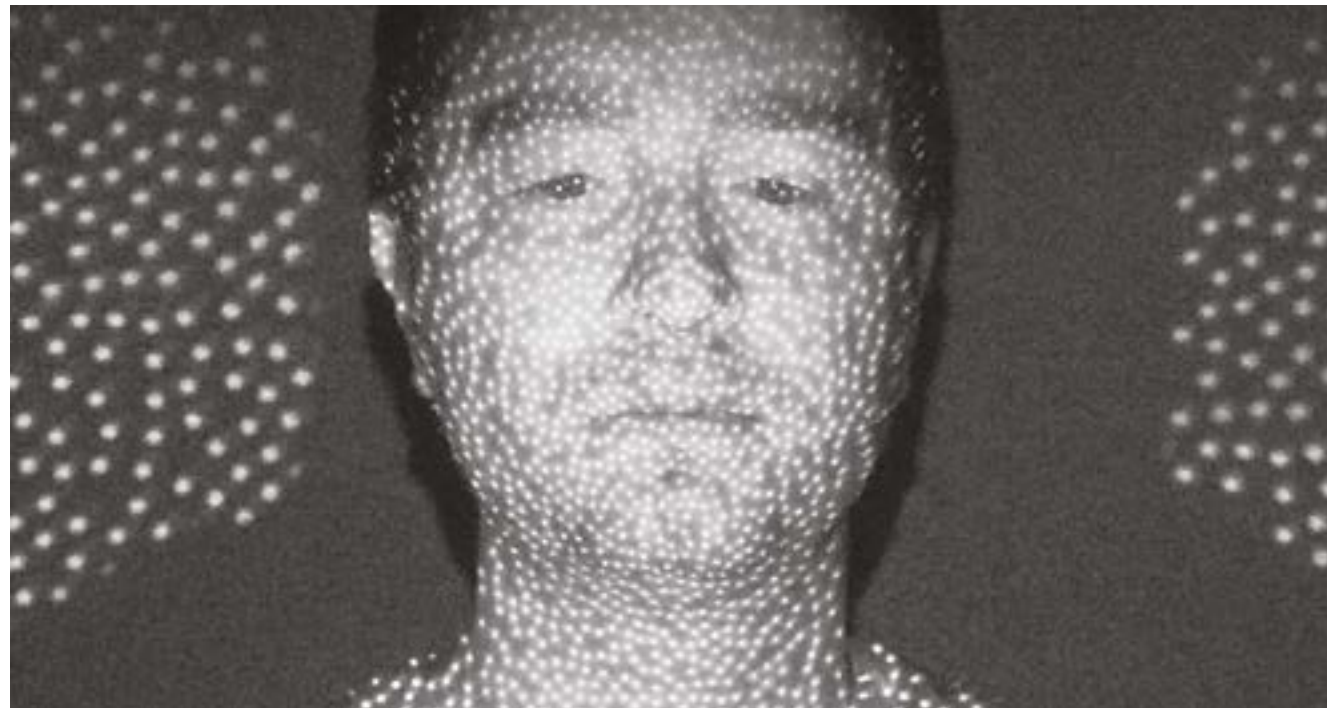
Apple's Face ID uses infrared scanning to let you sign in using just a snap of your face // Bloomberg
