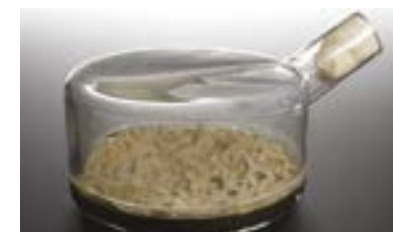
Thousands of glass fermentation vessels like this one were used in Glaxo (now GlaxoSmithKline) laboratories to produce penicillin. Photo Credit: Welcome Images
