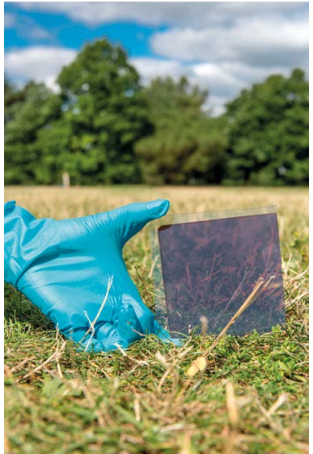
330nm-thick film of organometal halide perovskite fabricated on a glass sheet. This film is the active element of Perovskite 20% efficient solar cells. Photo credit: TheGuardian
