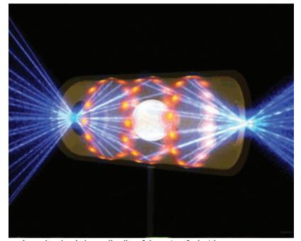
192 lasers bombarded a small pellet of deuterium fuel with an energy twenty times that of any previous experiment.
