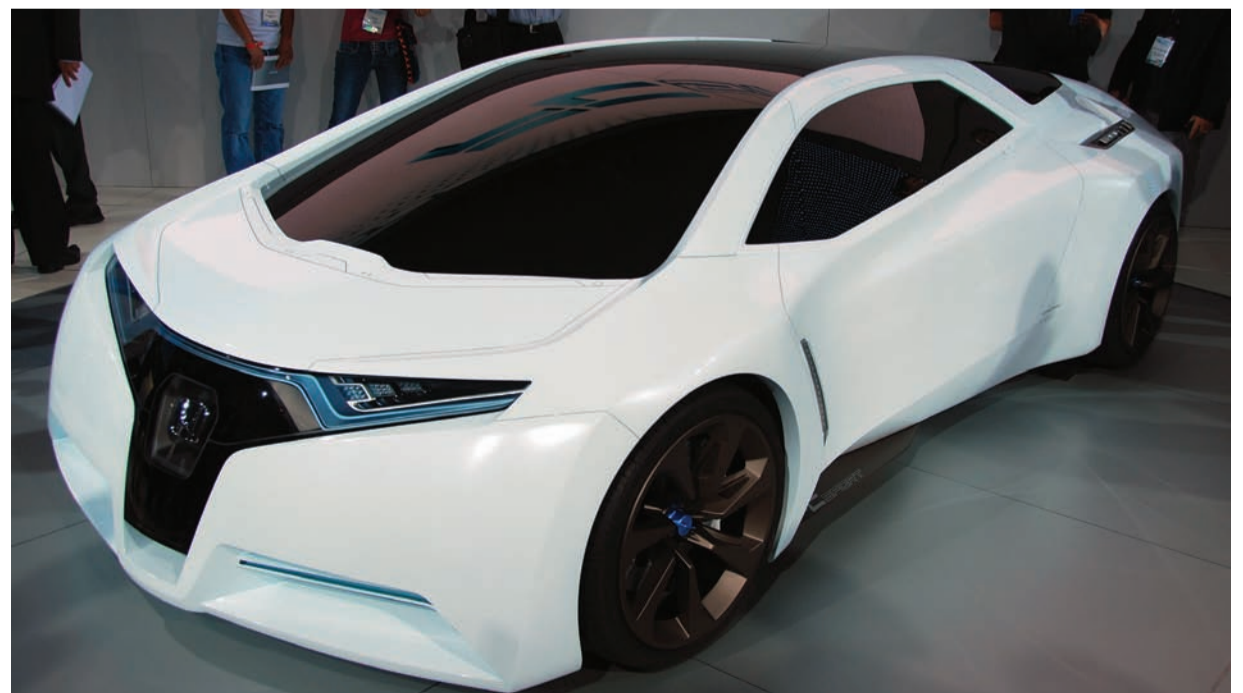
The Honda FC Sport Concept is a hydrogen fuel cell sports car with body panels made from bioplastics
