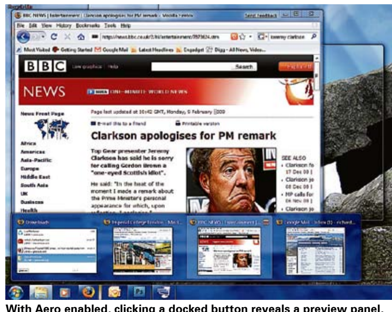
With Aero enabled, clicking a docked button reveals a preview panel, and hovering over a thumbnail highlights the associated window.
